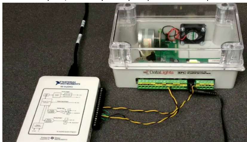
Figure 7 EPC and MyDAQ, Laboratory scenery for speed and thermal processes
