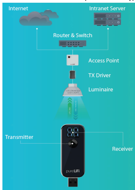
Figure 4 Connection Li-Fi devices (Li-Fi assembly)
